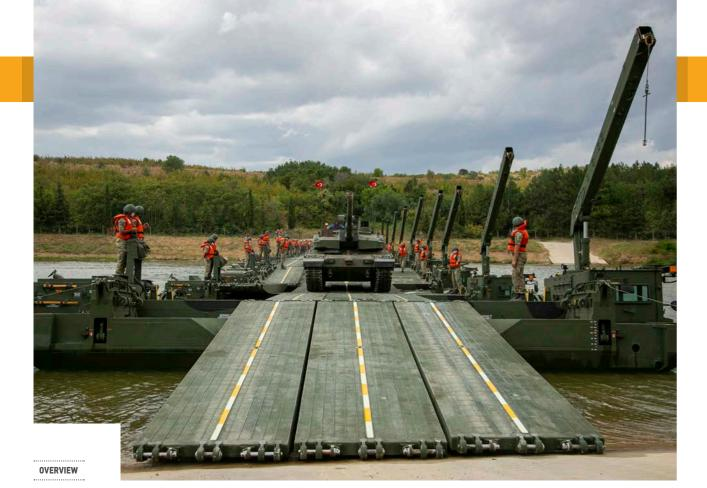
The OTTER is a bridge and ferry system designed for safe and fast transport of combat and logistic military vehicles in river crossing operations.
